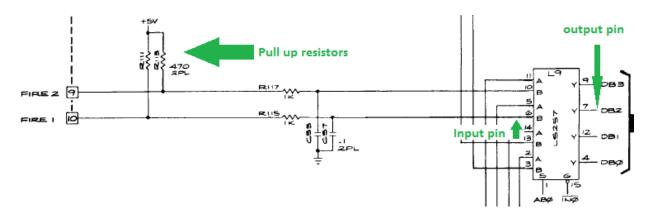
To test the inputs, first test the input to the pin, and verify it's high (+5V) when not pressed, and that it goes low when the button is pressed. If this happens you are good from the chip input to the button's switch and that switch is wired up correctly to ground. If you find that the input is normally LOW or that the input is normally HIGH, but never goes LOW, then physically check your button's microswitch and check that the wiring to the game board is OK.
